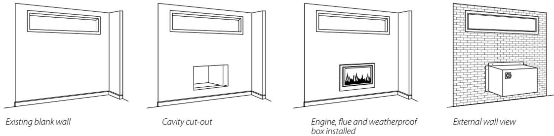
For an alternative installation to a false fireplace, the Rinnai 1250 & 950 can be installed into a weatherproof box. A cavity is cut into the existing blank wall and the fireplace is installed onto a bracket that allows the back of the fire to sit outside housed in a tightly sealed box. This option allows the fire to be built into an existing wall without taking up any extra space in the room. The weatherproof box is sold separately.
