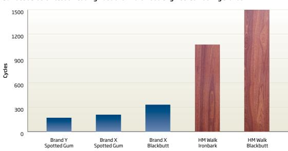
The abrasion test uses an abrasive on a wheel and measures the number of cycle revolutions that is required to wear through the coating to bare wood. The higher the number of cycles the more abrasive resistant the coating is to wear.
