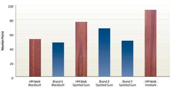
The dint test is the amount of force required to put a dint into the surface of the product. A higher number represents more force is required to dint the surface.
