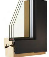
With a narrow aluminium strip on the sash, the Wood-Alu design presents a modern look, suitable for a range of applications. A revolutionary back-vented clip-on technique provides ventilation between the outer aluminium profile and the inner timber frame, therefore entending the durability of the window or door.
