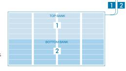
such that all blades in the top halves of all the bays form a bank and operate simultaneously and all the blades in the lower halves of all the bays form a second bank and operate simultaneously. However, various switching and wiring configurations allow multiple windows to be controlled simultaneously or independently depending on individual preferences.
