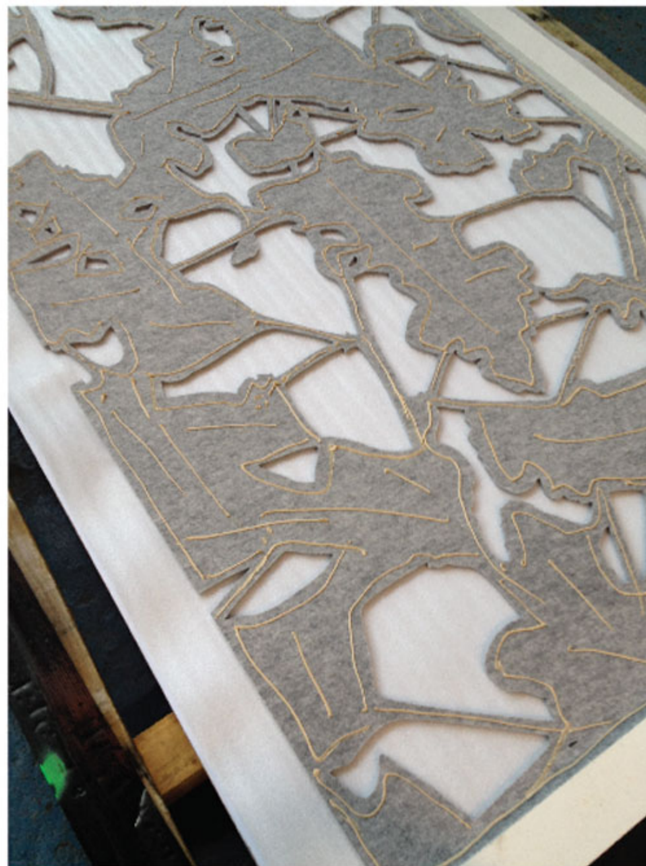
Applying Glue to laminate Screens (Application window - 20 mins!)
